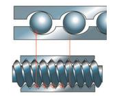
Notice many more contact points on the roller screw compared to the ball screw. This results in higher loadcarrying capacity and improved stiffness.
