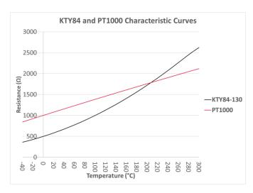
Figure 1. Characteristic Curves of KTY84 and PT100
