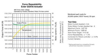
This data demonstrates the excellent force repeatability available to you in an open loop system. If your application requires even more accurate force control Exlar offers integrated force sensing devices for monitoring force in your application.
