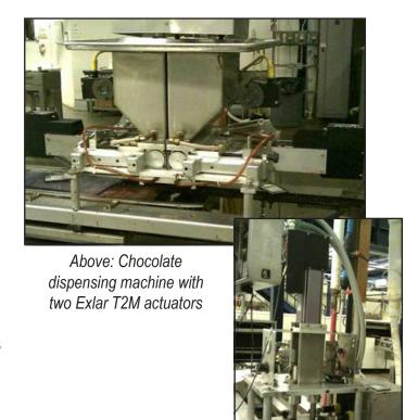
Pressing machine with an Exlar T2M actuator
