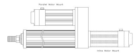
Figure 4: Motor Mounting Configurations
