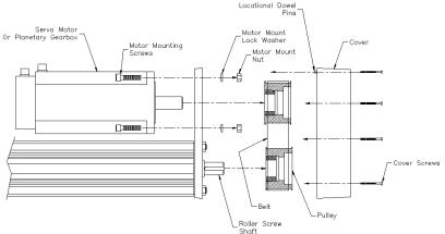
Figure 9: Parallel Motor Mount Drive Train Assembly\*
