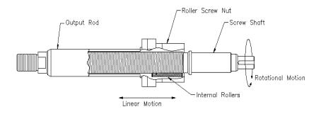
Figure 1: Actuator Operating Principle
