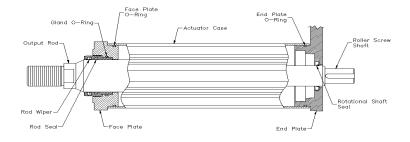
Figure 6: Actuator Sealing Details
