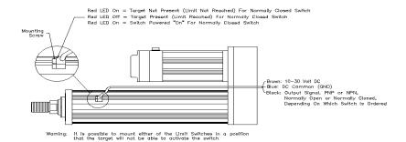
Figure 15A: Adjustable Limit Switch Wiring (FT35, FT60, FT80)
