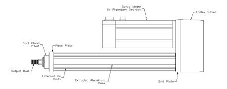
Figure 2: FT Actuator with Parallel Motor Mount
