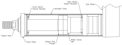
Figure 10: Actuator End of Stroke Cushions
