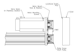
Figure 11: Parallel Motor Mount Disassembly
