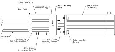
Figure 12: Inline Motor Mount Disassembly
