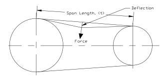
Figure 9: Belt Tension Diagram
