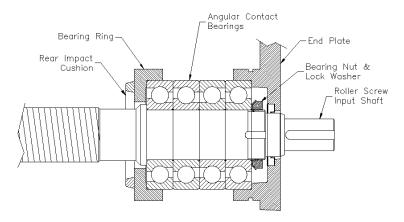
Figure 7a: Roller Screw Support Bearing Detail – FT35, FT60, and FT80
