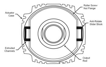
Figure 5a: Anti-Rotate Mechanism (FT35, FT60, and FT80)
