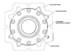
Figure 5b: Anti-Rotate Mechanism (FT45)
