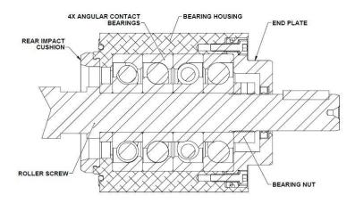
Figure 8: Roller Screw Support Bearing Detail - FT45
