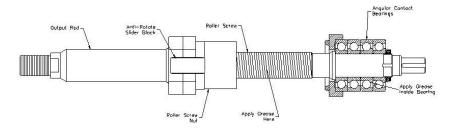
Figure 14a: Actuator Greasing Detail
