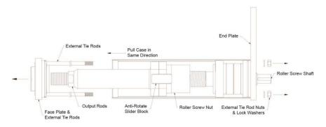
Figure 13: Actuator Disassembly
