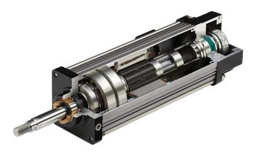
Electric actuators use roller screw technology, which enables high load capacity (more than 100,000 lb). Load capacity and rigidity of planetary roller screws suit applications requiring continuous force. Yet, these devices operate quietly, which helps in medical applications.
