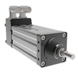
Integrated products (G-series) provide optimized power and connections to leading motion control systems with integrated servo motor and inverted roller screw technology
