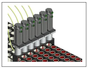
Exlar's GSX Series actuators directly operate piston pumps to fill cartons with liquid.
