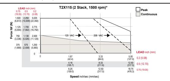
\*Test data derived using NEMA recommended aluminum heatsink 12" x 12" x 1/2" at 25°C ambient.
