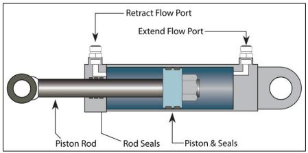
Figure 1- Basic Hydraulic Cylinder
