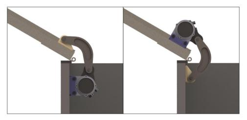
Figure 6 - Left: PH4 actuator in standard configuration; Right: PH4 actuator in "Follow-On" configuration.
