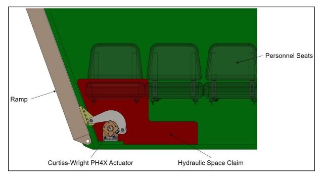
Figure 5 - Illustration showing space savings of a Curtiss-Wright PH4X REMA in place of hydraulics onboard an Armored Personnel Carrier.
