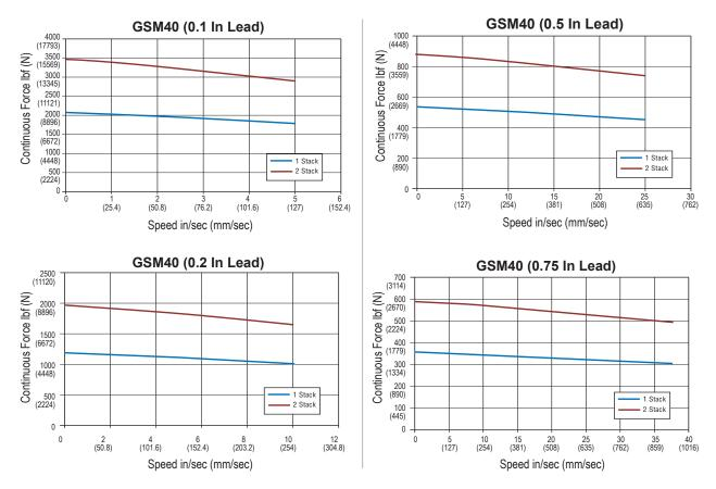
Test data derived using NEMA recommended aluminum heatsink 12" x 12" x 1/2" on GSM40
