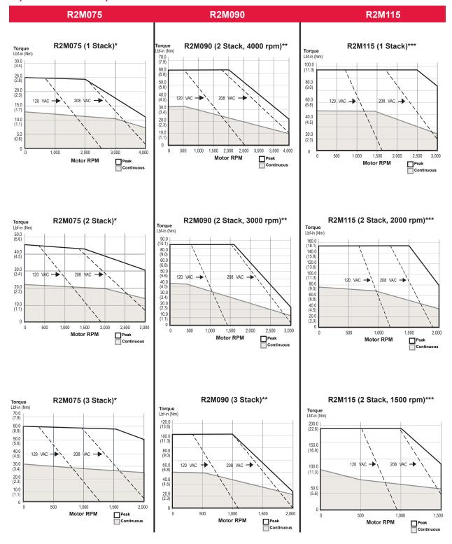
For R2G gearmotors, multiply torque by gear ratio and efficiency. Divide speed by gear ratio efficiencies; 1 Stage = 0.91, 2 Stage = 0.86
