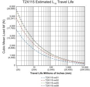
The  $L_{_{10}}$  expected life of a roller screw linear actuator is expressed as the linear travel distance that 90% of properly maintained roller screws are expected to meet or exceed. For higher than 90% reliability, the result should be multiplied by the following factors:  $95\% \times 0.62$ ;  $96\% \times 0.53$ ;  $97\% \times 0.44$ ;  $98\% \times 0.33$ ;  $99\% \times 0.21$ . This is not a guarantee; these charts should be used for estimation purposes only.
