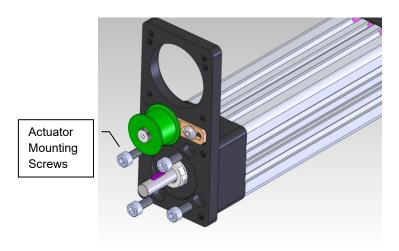
4 Place the key in the actuator shaft keyway. Clamp the actuator shaft pulley and tighten the actuator shaft pulley nut. See Section 3.9 Fastener Torque Values. See figure below.
