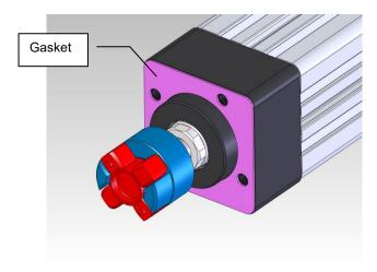
5 Place the inline housing over the pilot feature of the end cap. Take care to make sure that the correct end of the inline housing is mated with the inline gasket and end cap otherwise the mounting holes will not line up. See figure below.
