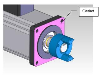
12 Insert the shaft of the motor into the inline housing with the motor coupling aligned to mate with the actuator coupling. Slide the motor in so the motor gasket and face plate flange is flush with the inline motor adapter plate pilot face. See figure below.
