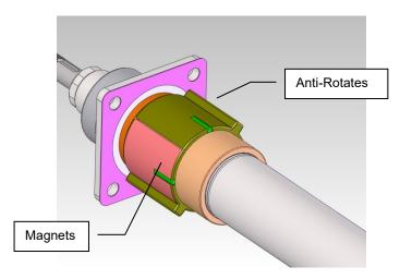
8 Slide the extend impact bumper over the main rod. See figure below.
