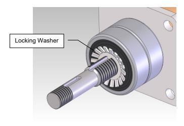
5 Torque the bearing lock nut onto the screw shaft and lock down a tang on the locking washer into the closest aligning notch on the bearing lock nut. See Section 3.9 Fastener Torque Values. See figure below.
