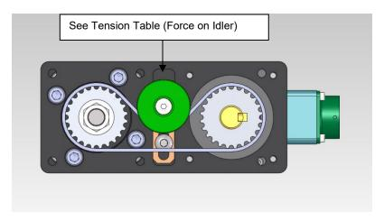
The idler pulley plate slot allows moving the idler pulley so the belt can be placed, followed by placing a force directly over the idler pulley to obtain the proper tension to tighten the belt (See table next page).
