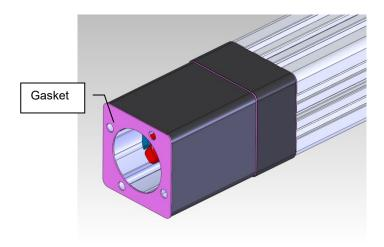
7 Place the inline motor adapter plate so it pilots into the inline housing. See figure below.
