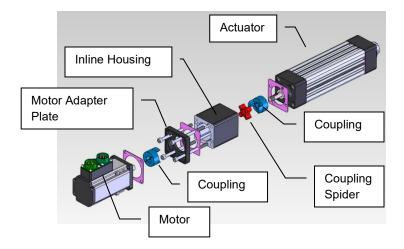
Figure: Inline Motor Mount Drive Train Assembly
