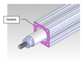
16 Slide the face plate over the main rod and gently tap the face plate until the rod wiper rides onto the main rod. Once the wiper seal is over the main rod continue to slide toward the case until it is flush with the case and gasket. See figure below.
