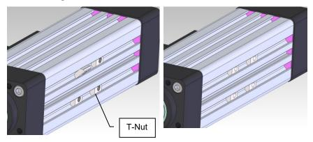
Step 1: Insert T-nuts at an angle into the t-nut rail slot.
