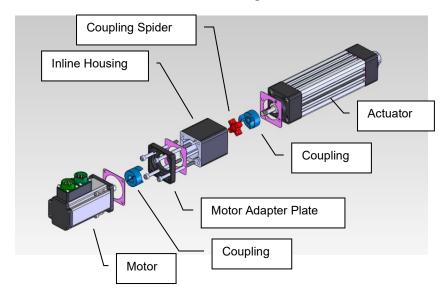
Figure 12: Inline Motor Mount Disassembly
