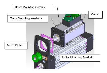
8 Remove the actuator mounting screws and remove actuator and gasket. See figure below.
