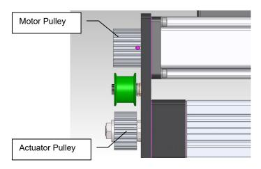
9 Install and tension timing belt. See Belt Tensioning below.
