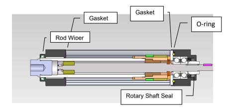
Figure: Base Unit Sealing Details
