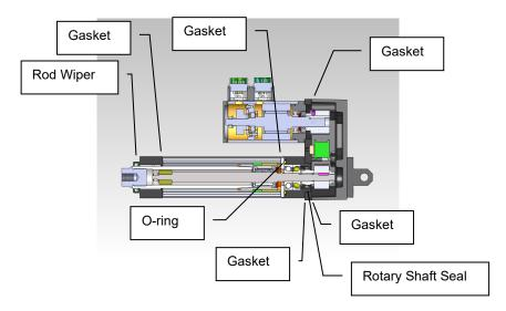
Figure: Parallel Motor Mount Unit Sealing Details
