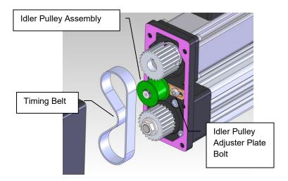
6 Loosen the set screws on motor pulley and slide the pulley off the shaft. Clamp the actuator shaft pulley and loosen actuator shaft pulley nut and remove. Slide the pulley off the actuator shaft. Take care not to lose the keys for each shaft. See figure below.
