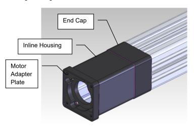
8 Insert the 4 inline housing screws and tighten to the designated torque value. (See table in Section 3.9). See figure below.
