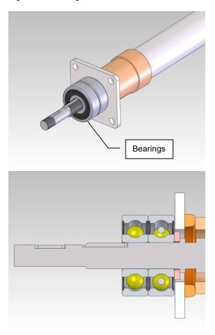
4 Place the locking washer onto the screw shaft. Make sure that the inner tang on the locking washer is placed into the keyway. See figure below.
