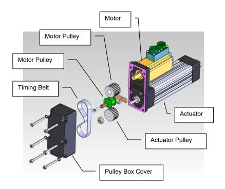
Figure: Parallel Motor Mount Drive Train Assembly
