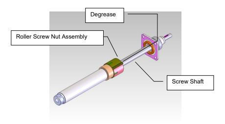
**Lubrication**—The planetary roller screw shaft or acme screw shaft and nut assembly, anti-rotates, linear bearing, and rotary seal are factory lubricated. The anti-rotate and linear bearing does not need relubrication. If the roller screw shaft or acme screw shaft need relubrication, follow the disassembly process for the actuator in Section 3.8 Disassembly & Reassembly Procedure.
