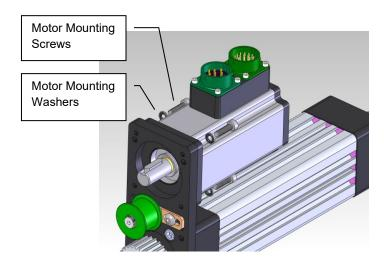
8 Place the key in the motor shaft keyway. Slide the pulley on and align it with the screw shaft pulley. Once aligned, torque the pulley set screws. See Section 3.9 Torque Values. See figure below.
