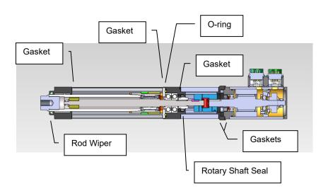
Figure: Inline Motor Mount Unit Sealing Details
