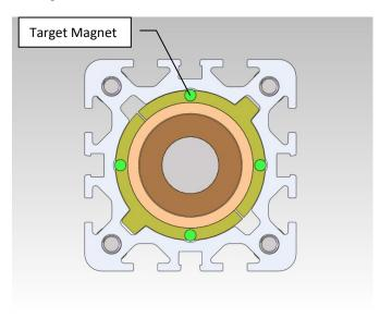
The limit switches are available with normally open and normally closed output, channel mount magnetic sensing prox.
