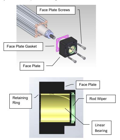
2 Loosen and remove the end cap screws and slide the end cap off the bearings. You will then be able to remove the o-ring from the end cap. Note: A shaft seal is used on KT actuators and can then be removed from the end cap if it needs to be replaced. See figure below.
