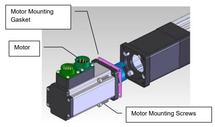
4 Loosen and remove screws from the motor adapter plate and inline housing. See figure below.
