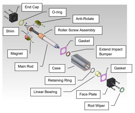
Figure: Actuator Disassembly
