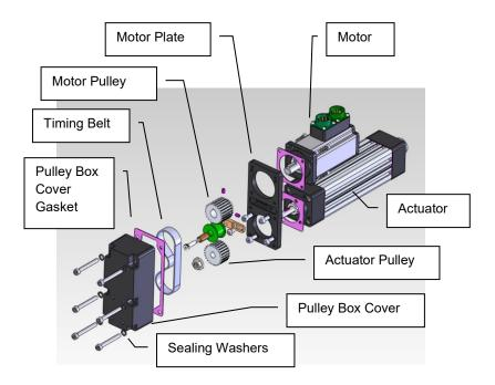
Figure: Parallel Motor Mount Drive Train Assembly
