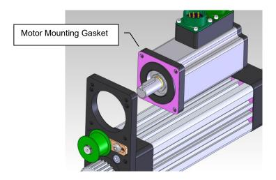
6 Place the motor output shaft through the output shaft hole on the motor plate until the motor gasket and motor face plate face are flush against the motor plate pilot face. See figure below.
