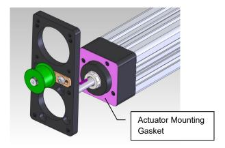
2 Place the actuator input shaft through the actuator hole on the motor plate until the actuator gasket and actuator face plate are flush against the motor plate pilot face. See figure below.
