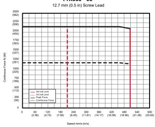
\*Test data derived using NEMA recommended aluminum heatsink 10" x 10" x 3/8" at 25 °C ambient.
