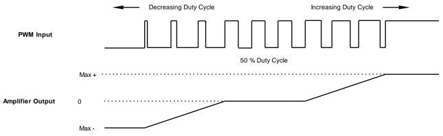
The command can be inverted so that increased duty cycle commands negative output and vice versa.
