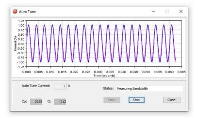
• A set of Cp and Ci alternatives, and the bandwidth measured using the high Cp and Ci values are displayed.
