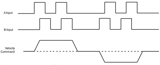
The ratio can be programmed for electronic gearing.
