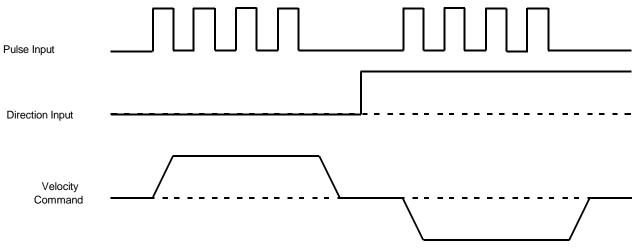
The amplifier can be set to increment position on the rising or falling edge of the signal. Stepping resolution can be programmed for electronic gearing.
