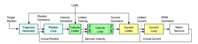
In velocity mode, the velocity loop drives the current loop. In current mode, the current loop is driven directly by external or internal current commands.
