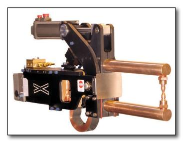
To meet ever-increasing production demands, automation engineers in the automotive industry have increasingly turned to electromechanical actuation solutions to improve their spot welding capability. A typical alternative is the electromechanical actuator based on ball or roller screw technology.
