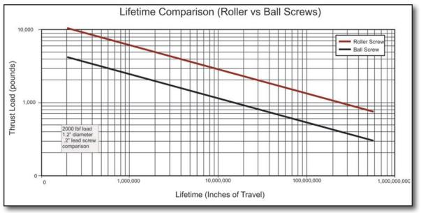
The Estimated Travel Life Comparison Between a Ball Screw and a Comparably Sized Roller Screw for a Given Load
